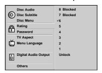
You cannot play DVD discs rated higher than the level you select unless you cancel the parental lock function. For example, when you select level 6, discs rated higher than level 6 are blocked and cannot be played.
